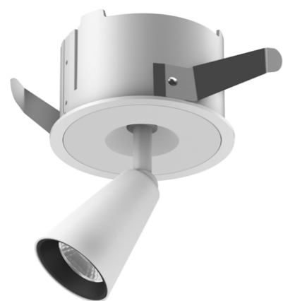
Model: MSTY-RM0805-Framed Power: 8W Cutout: Ø94mm Size(WxLxH): Ø100X109mm
